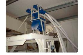
**RATAJ®** flexible shaftless screw conveyors (types SL, SLK, SLN, SLP) are used for the transport of fine and light materials with transport performances from about 0.001 to 15 m³/hr. A major advantage of these conveyors is the possibility of transport in curves and over
