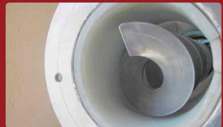
**Basalt** is used for the transport of abrasive materials or for conveyors which operate also without material. The 20mm thick basalt inserts are of through or circular design. They are mainly used in power and mining industry for the transport of ash, slag, coal and other abrasive materials.
